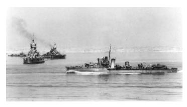
Prior to its sinking, there had been plans to re-gun the ship with the same guns used by the G and H-class destroyers she was based on. This was due to the finite amount of ammunition for the guns and the lack of spares as the guns wore out. The 3.7cm AA guns had been replaced with 20mm Oerlikons in 1941 for the same reason as well as an effort to save weight.
